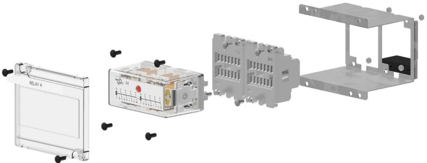
Figure 6: Exploded view of the size 4 element kit
